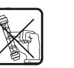
**GR** Halogen lamps must not be contacted with the hands. It is preferable to use a clean, dry cloth.
