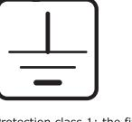
**GR** Protection class 1: the fitting must be earthed.
