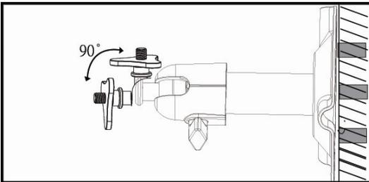
Loosen up the Thumb screw.
