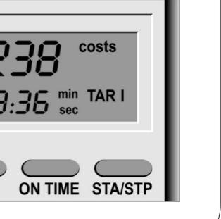
M12 IT's standard function indicates the consumption of a connected device. The calculator indicates the relevant costs of 2 tariffs can be set. The start screen (1) appears automatically after plugging the device in a wall socket. The device is connected directly to M12.
