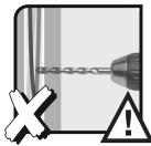
**WARNING** Be careful when drilling to ensure no cables or pipework may be affected. **Ensure correct drill is used suitable** for wall fixings
