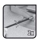
5. Attach the device onto the wall bracket, check the angle of the device is suitable and tighten the fixings using the Hex key provided.
